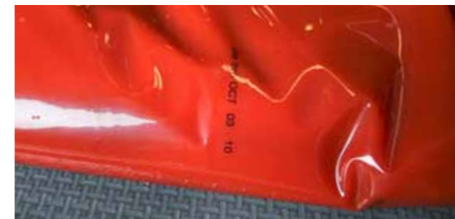
Date marking of bags for large scale catering with an Allen 53Li
