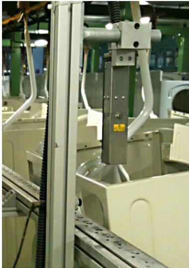
Especially the heavy work environment has led SIA to the choice of Hitachi Inkjet Printer products. The printer works properly and efficiently under high temperature changes with automatic regulation of ink viscosity.
